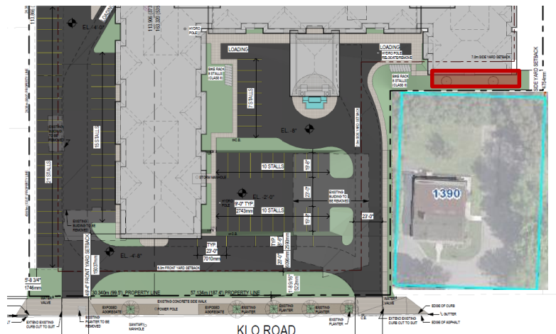
Figure 1 – The area noted in red indicates the requested side setback variance from 7.0 m required to 4.5 m proposed.
