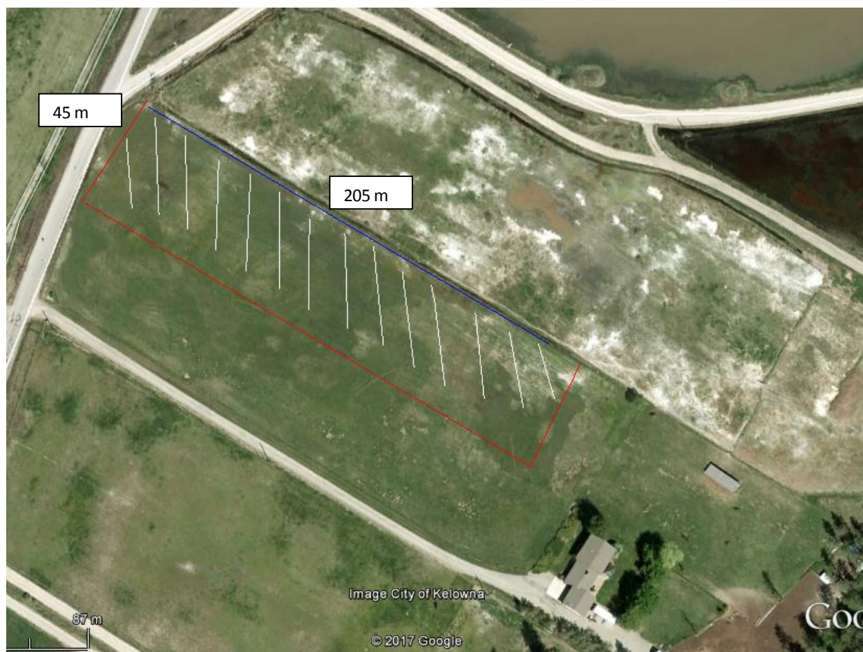
Figure 1. 841 Curtis Rd. The red lines mark the area to be improved with fill, the white lines represent the lateral drainage trenches at 10 m spacing and the blue line is the constructed ditch on the north side of the property.
