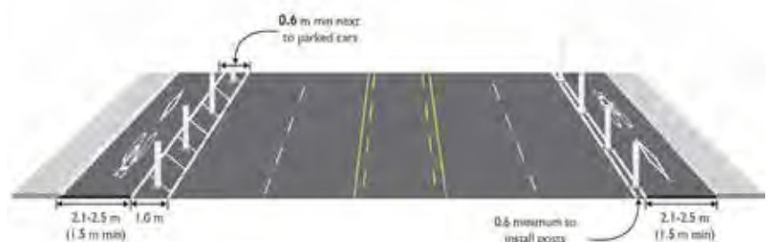
Figure 6.13: Retrofit Cycle Track Configurations
