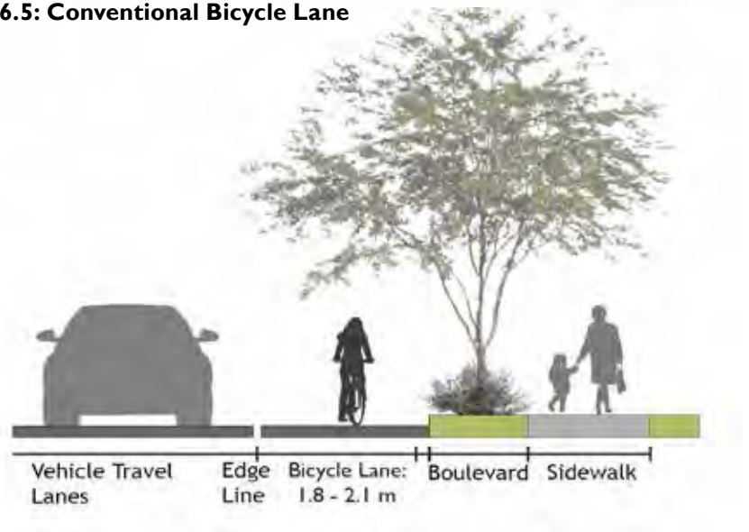
Figure 6.5: Conventional Bicycle Lane
