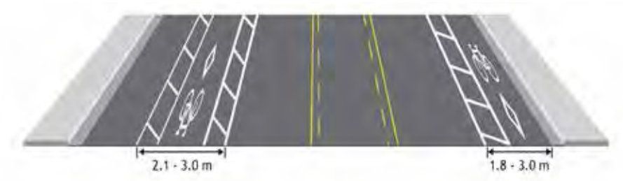
Figure 6.7: Buffered Bicycle Lane
