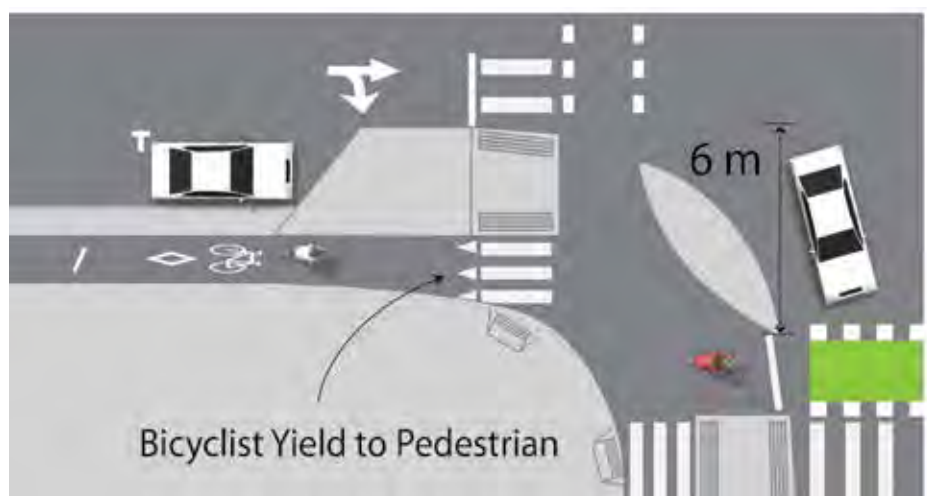
Figure D.2: Cycle Track at a Corner Refuge Island
