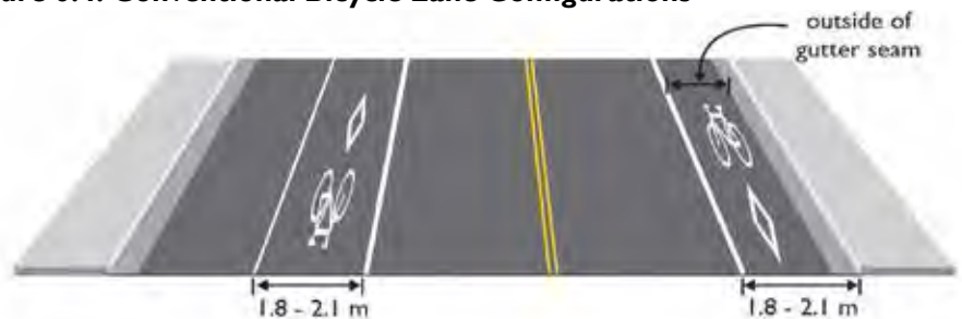
Figure 6.4: Conventional Bicycle Lane Configurations
