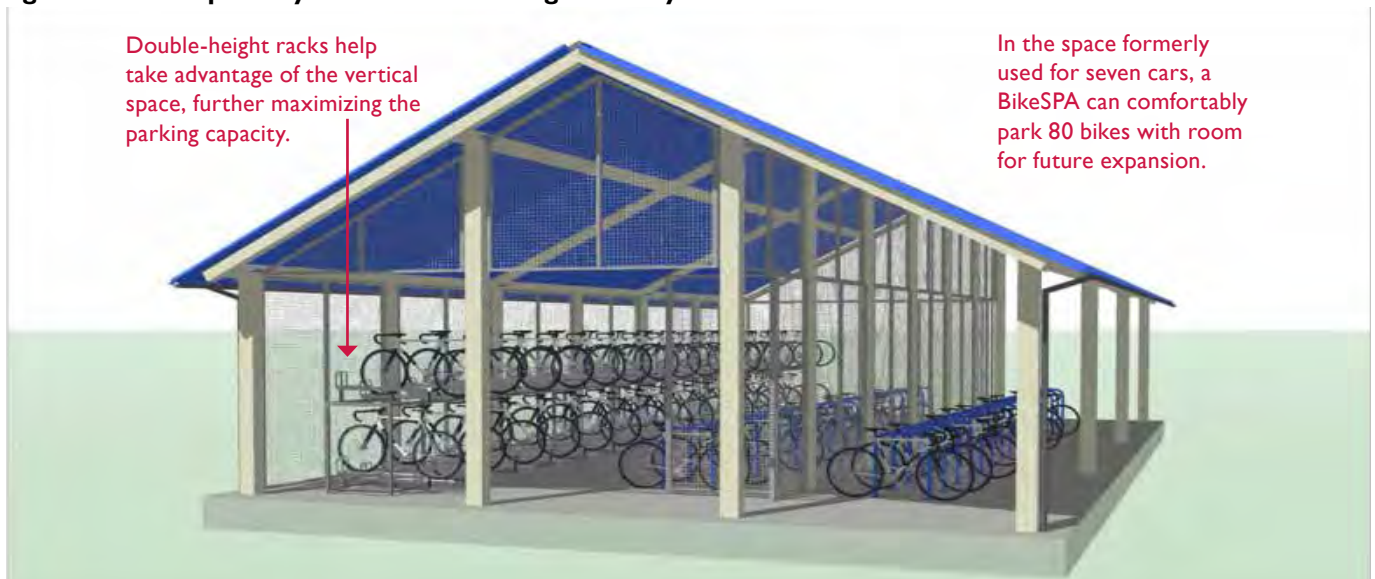
Figure 6.17: Sample Bicycle Secured Parking Area layout
