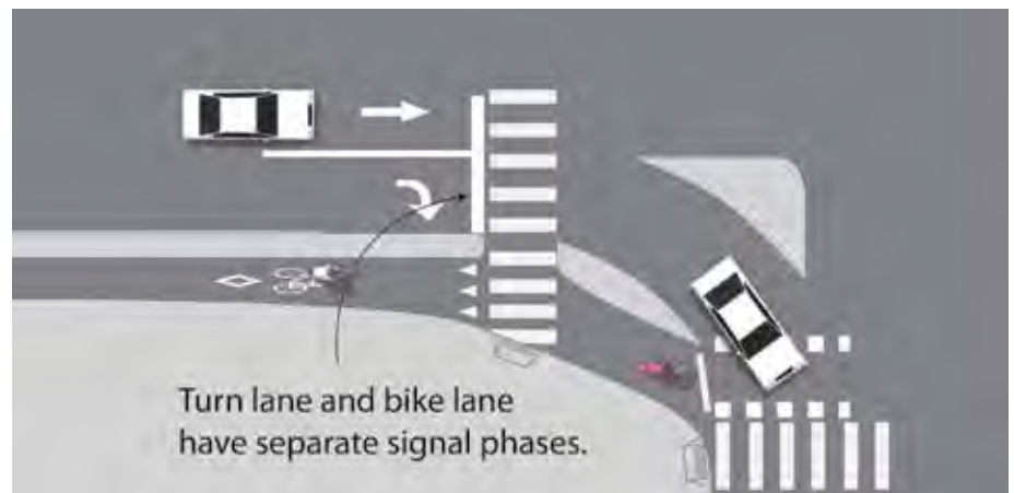
Figure D.6: Signalized Refuge Island
