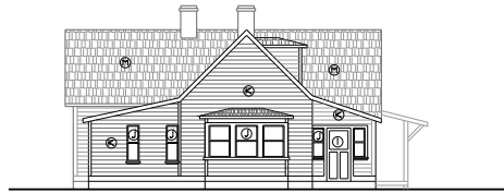
EXISTING WHITE HOUSE - NORTH ELEVATION SCALE: 1/8" = 1'-0"
