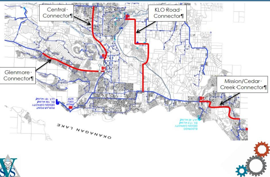
Construct an agricultural water transmission system that provides redundancy and resiliency for distributing source water supply the distribution system
