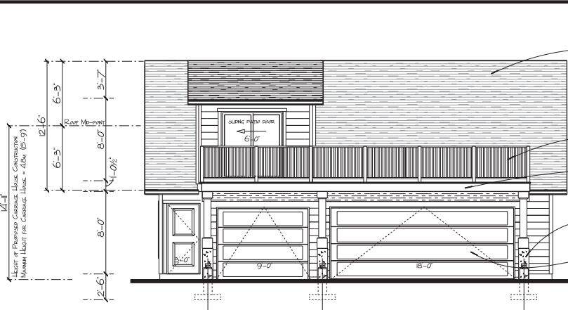
CARRIAGE HOUSE FRONT ELEVATION SCALE: 1/4" = 1'-0"
