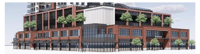
The applicant is seeking to increase the height of the podium to maximize the first level to be activated with commercial retail units and the second level to be predominantly office space. Limited vehicular parking begins on the second level and carries to level five. The applicant has designed the over height podium with
