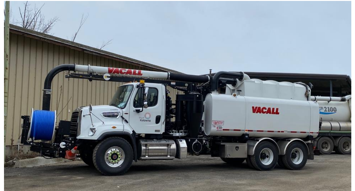
Vac-Truck used to regularly to clean out Catch Basins and drains
