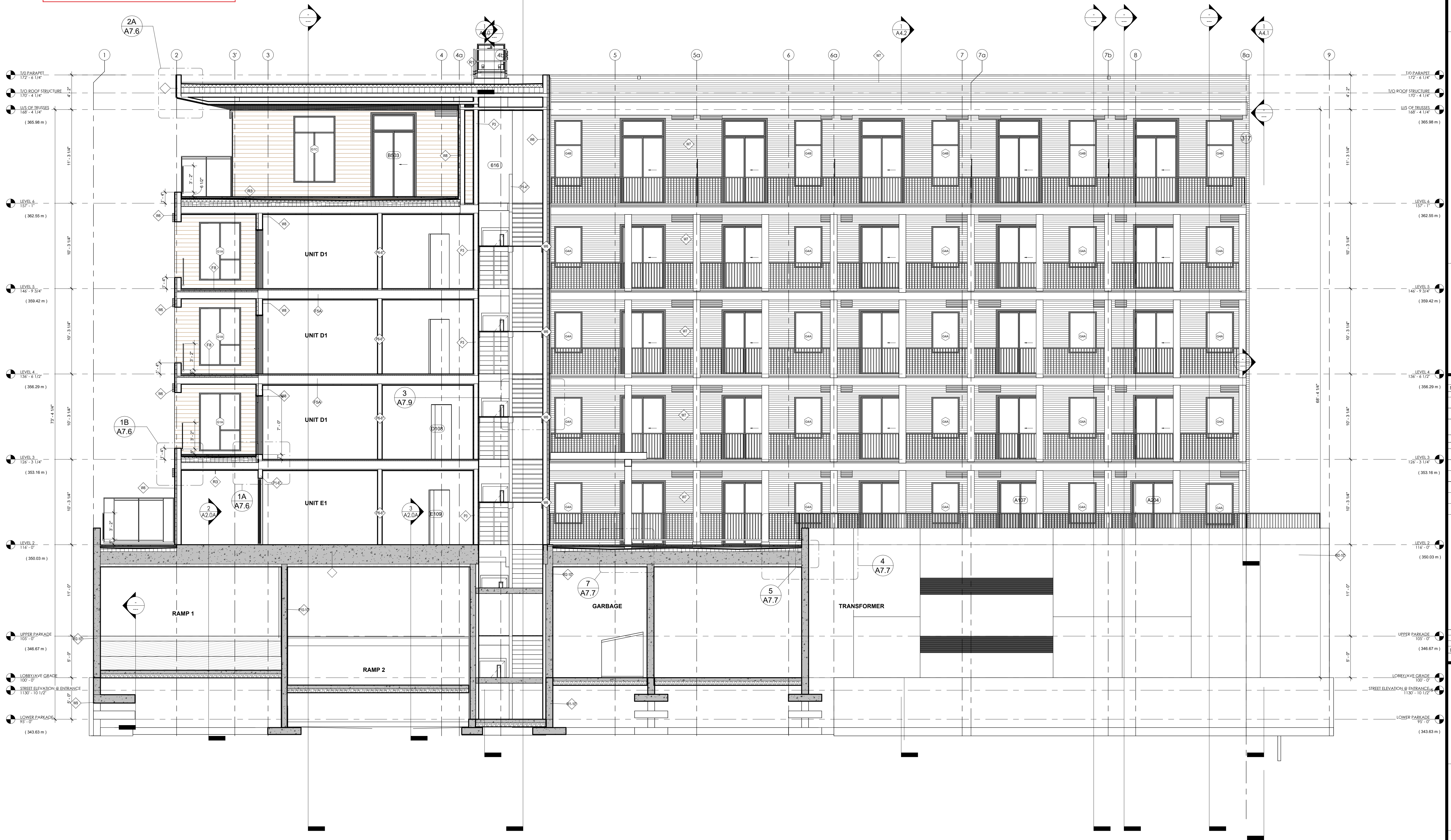
1 A4.3 BUILDING SECTION - EAST/WEST 3/16" = 1'-0"
