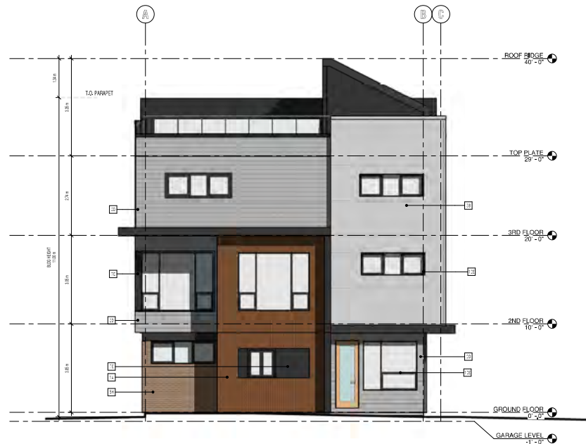
1 INTERIOR SIDE ELEVATION 1/4" = 1'-0"
