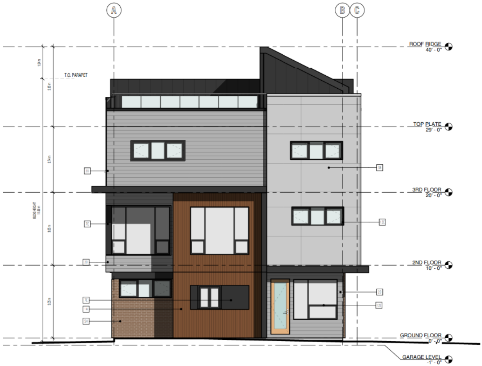
1 INTERIOR SIDE ELEVATION A-3.2 1/4" = 1'-0"
