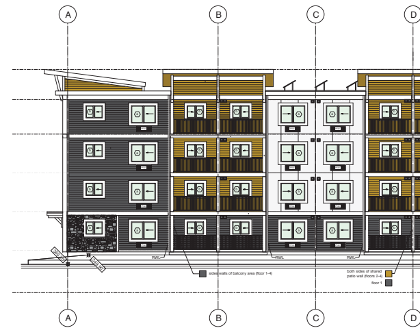
2 Building B - West Elevation - North End 1/8"=1'-0"
