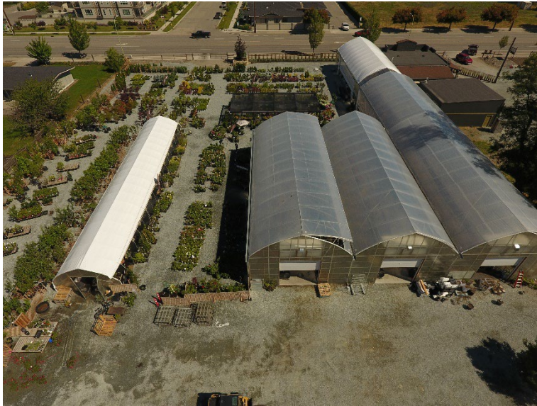
Figure 2. Aerial image captured June 2024 facing north of gravel installed on top of previous parking area and landscaping fabric to support container nursery production and winter plant storage.
