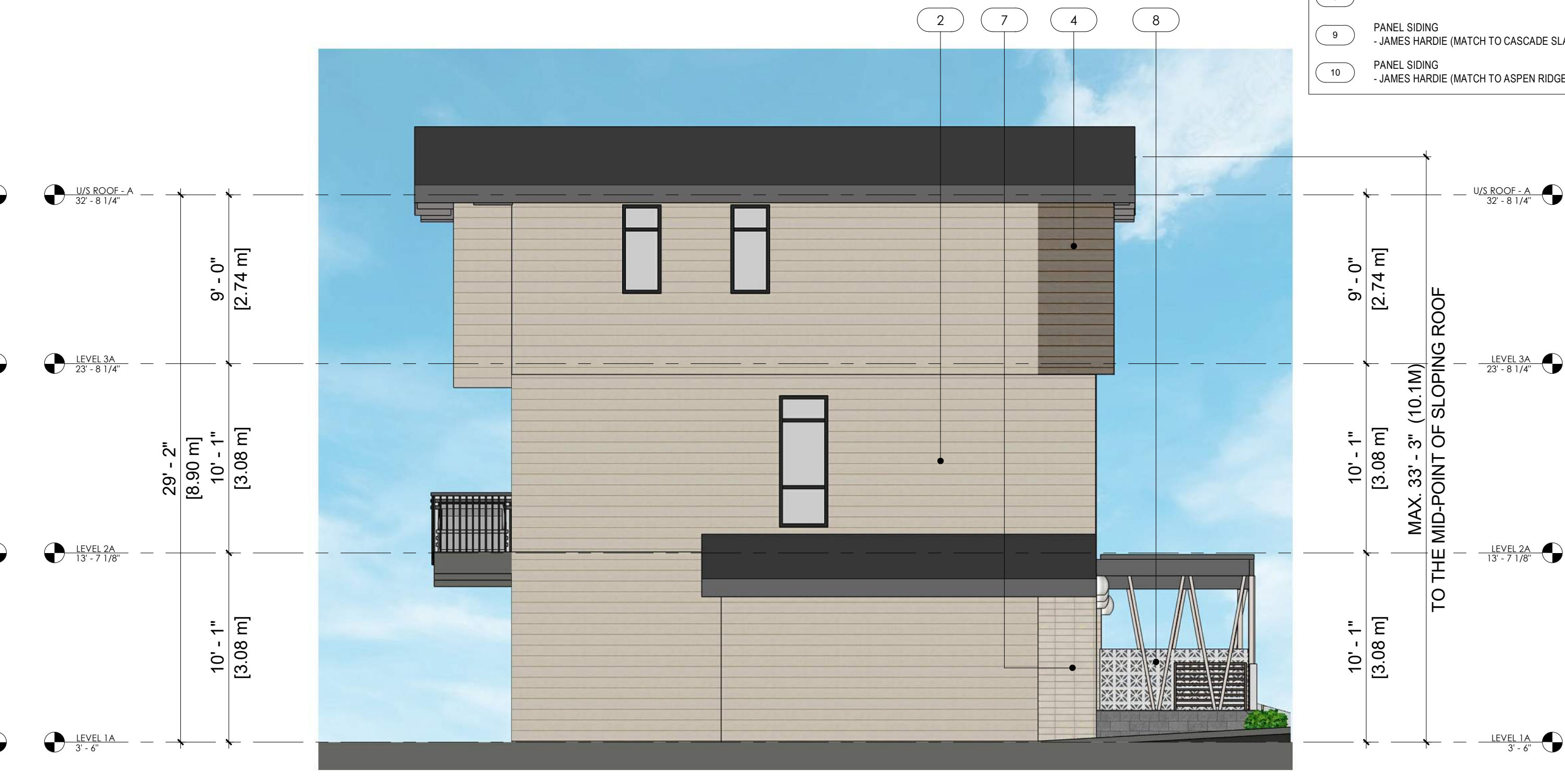
2 WEST ELEVATION - UNIT #1-#4 A3.2 3/16" = 1'-0"
