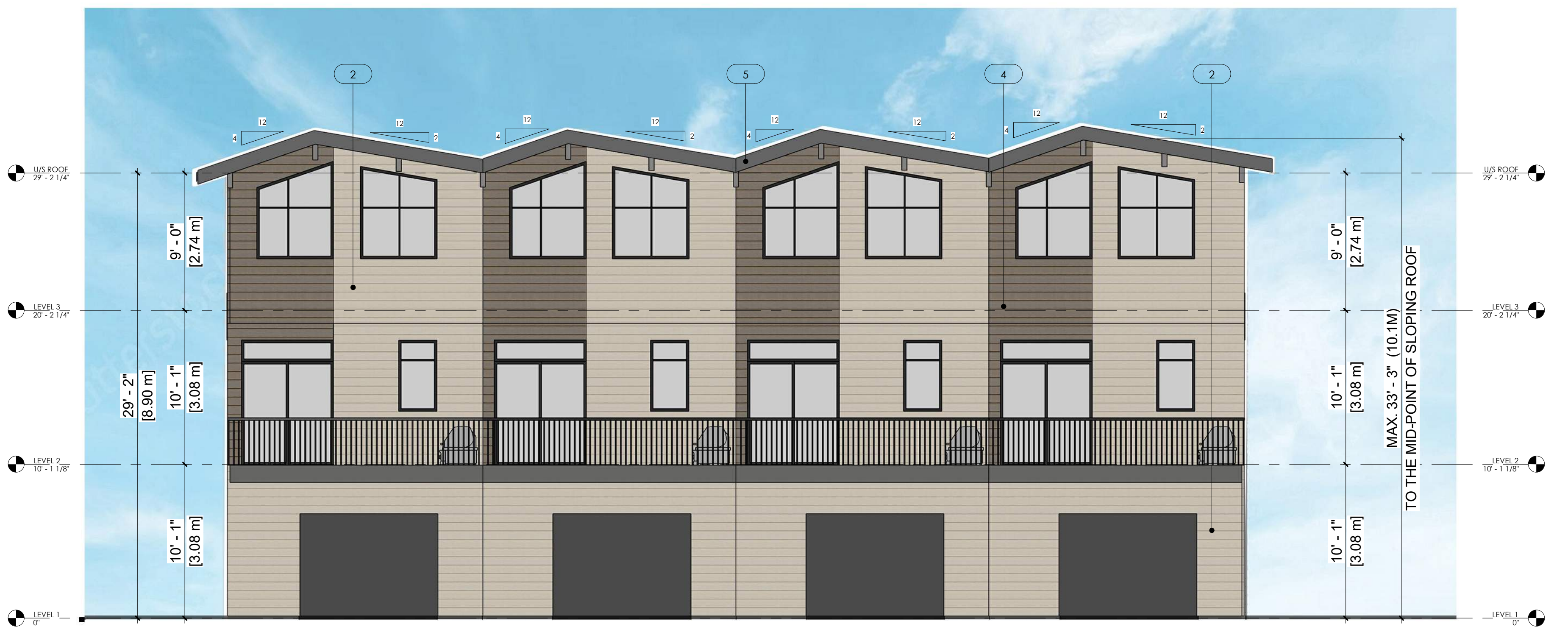
1 EAST ELEVATION - UNIT #11-#14 A3.3 3/16" = 1'-0"
