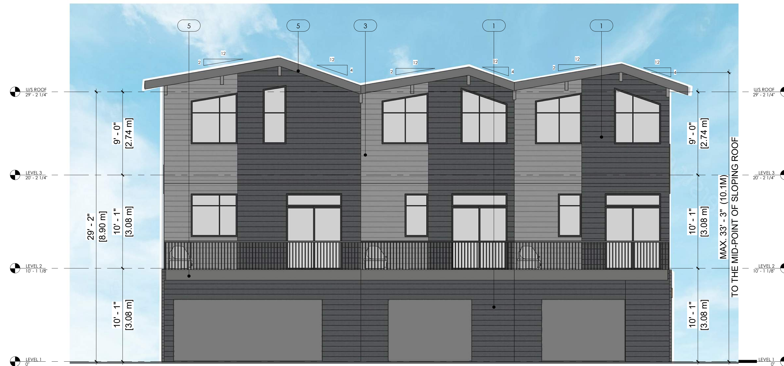
2 WEST ELEVATION - UNIT #15-#17 A3.4 3/16" = 1'-0"
