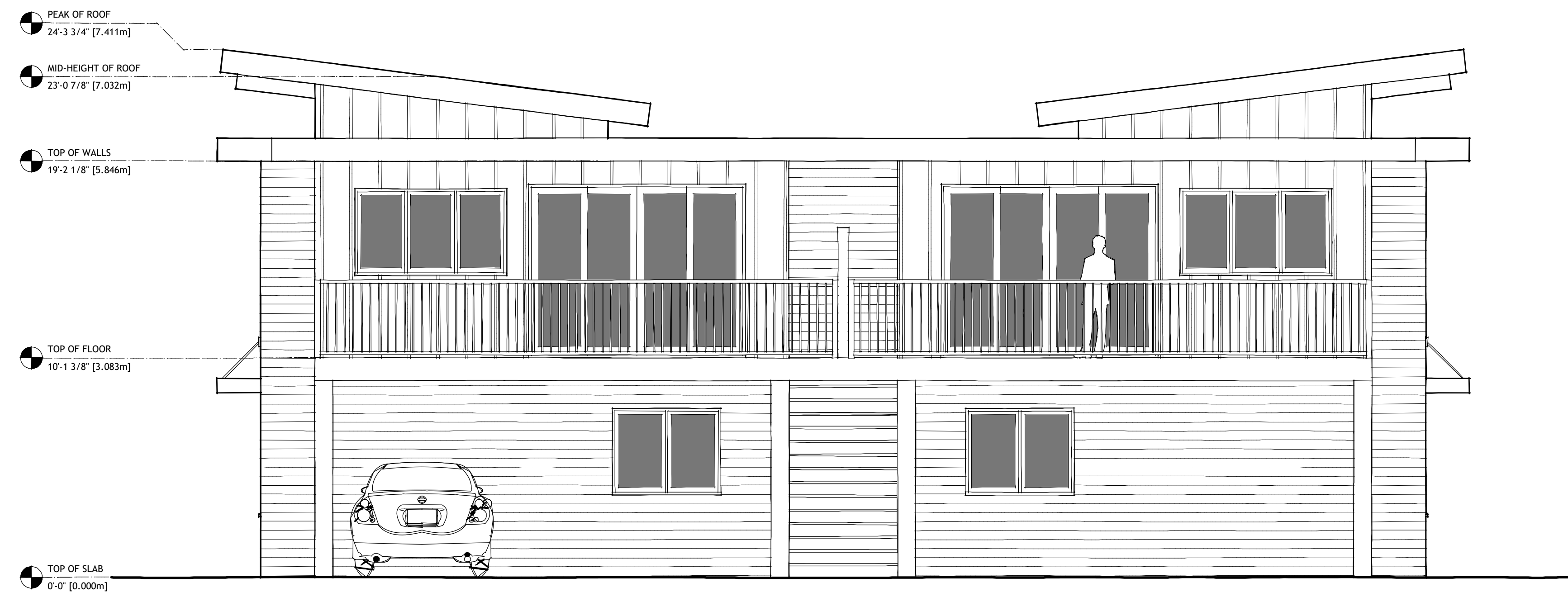
2 WEST ELEVATION Scale: 1/4" = 1'-0"
