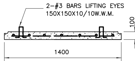
BOTTOM SLAB DETAIL
