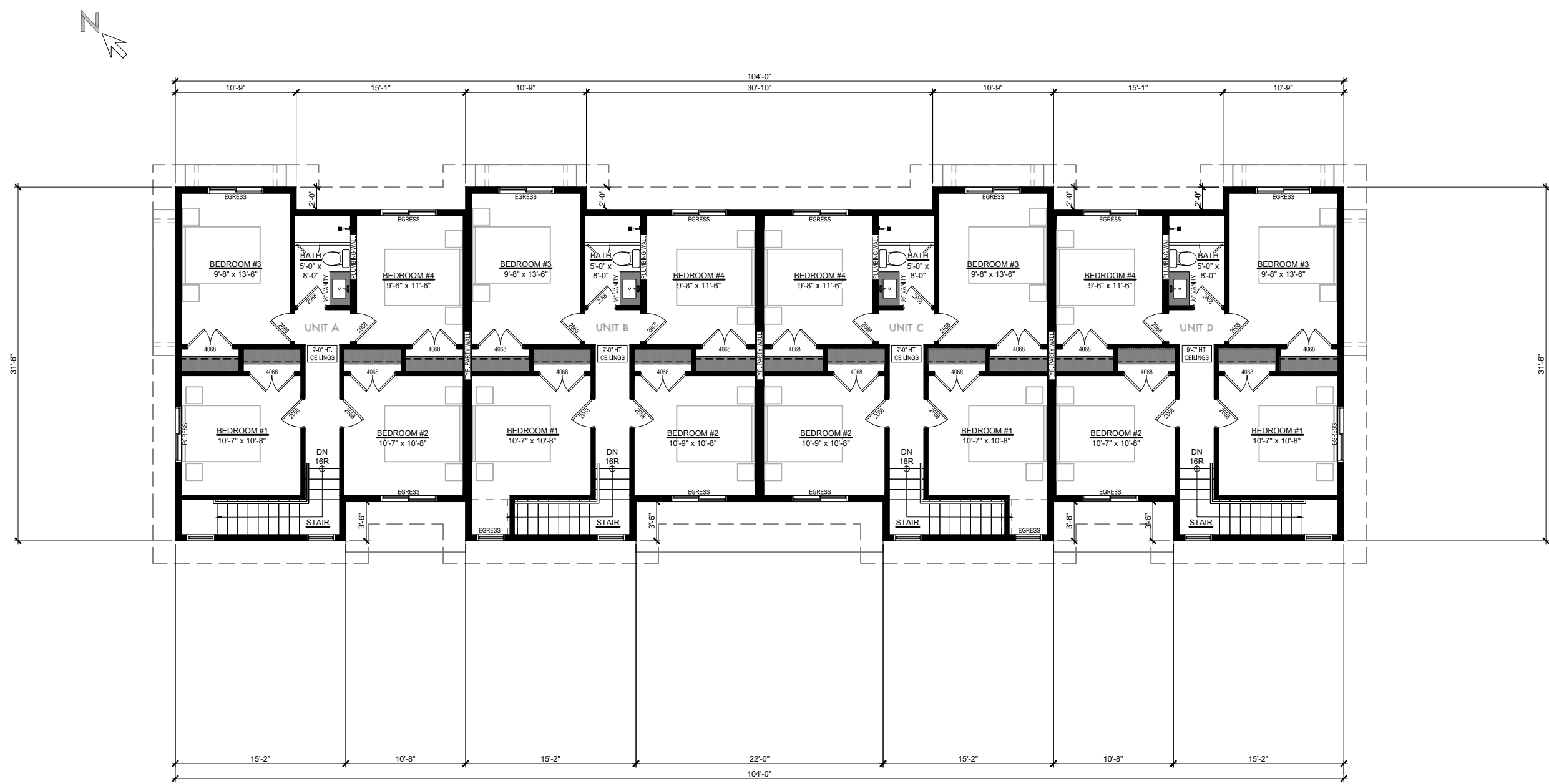
UPPER FLOOR PLAN 3/32" = 1'-0" FLOOR AREA - UNIT A: 685 SqFt FLOOR AREA - UNIT B: 700 SqFt FLOOR AREA - UNIT C: 700 SqFt FLOOR AREA - UNIT D: 685 SqFt
