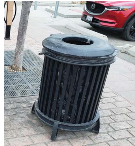
Figure 24: Chipping of powdercoat along rim of waste receptacle
