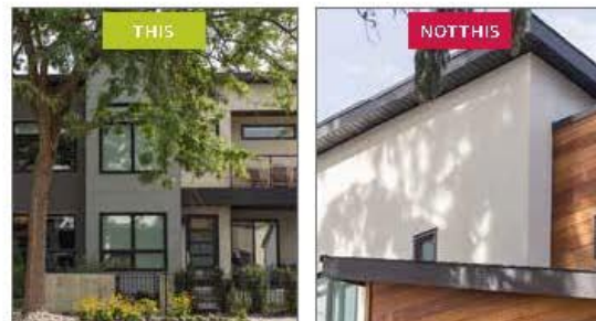
Figure 28: Front doors should be directly accessible via a walkway, porch and/or stoop, and front yards should incorporate complementary landscaping and modest fencing (3.3.1 c, d).
