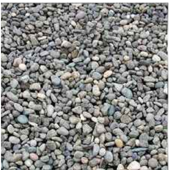
ROOFING MATERIAL GRAVEL BALLAST
