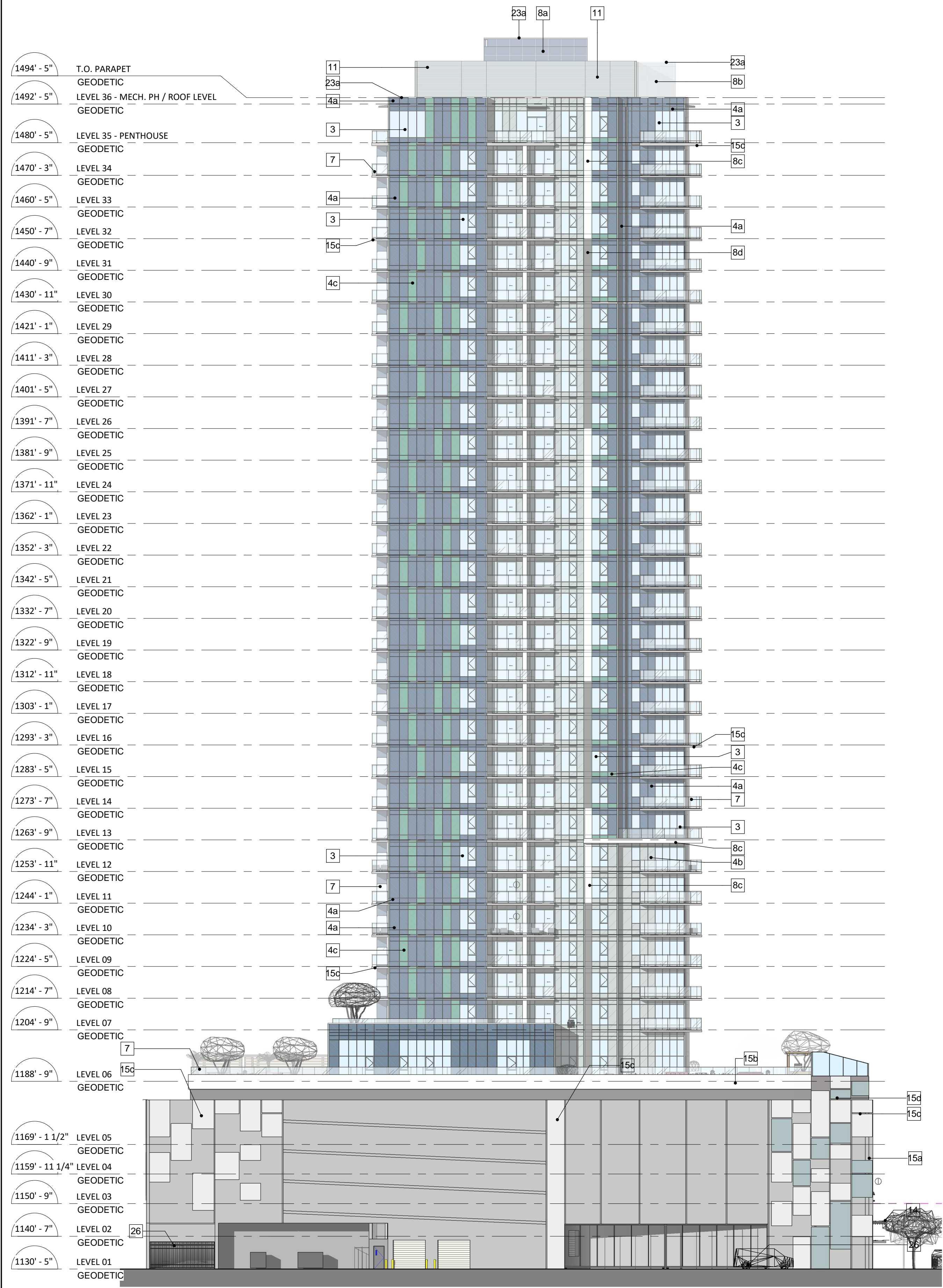
1 OVERALL EAST ELEVATION DP2.02 Scale: 1 : 250
