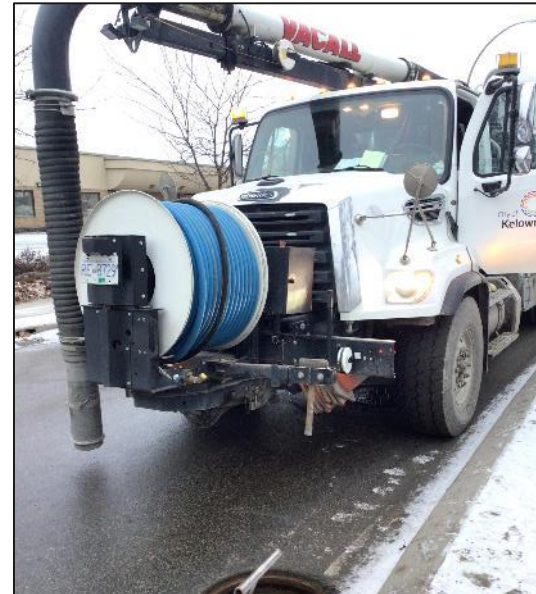
Vacuum trucks for cleaning and flushing
