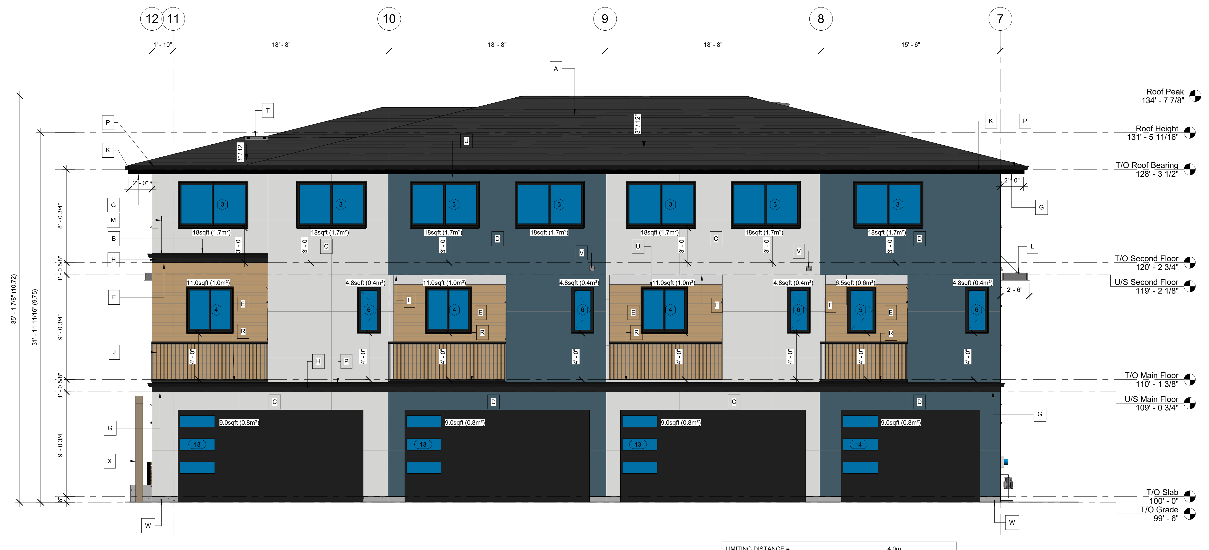
1 BLDG 2 - EAST ELEVATION 1/4" = 1'-0"
