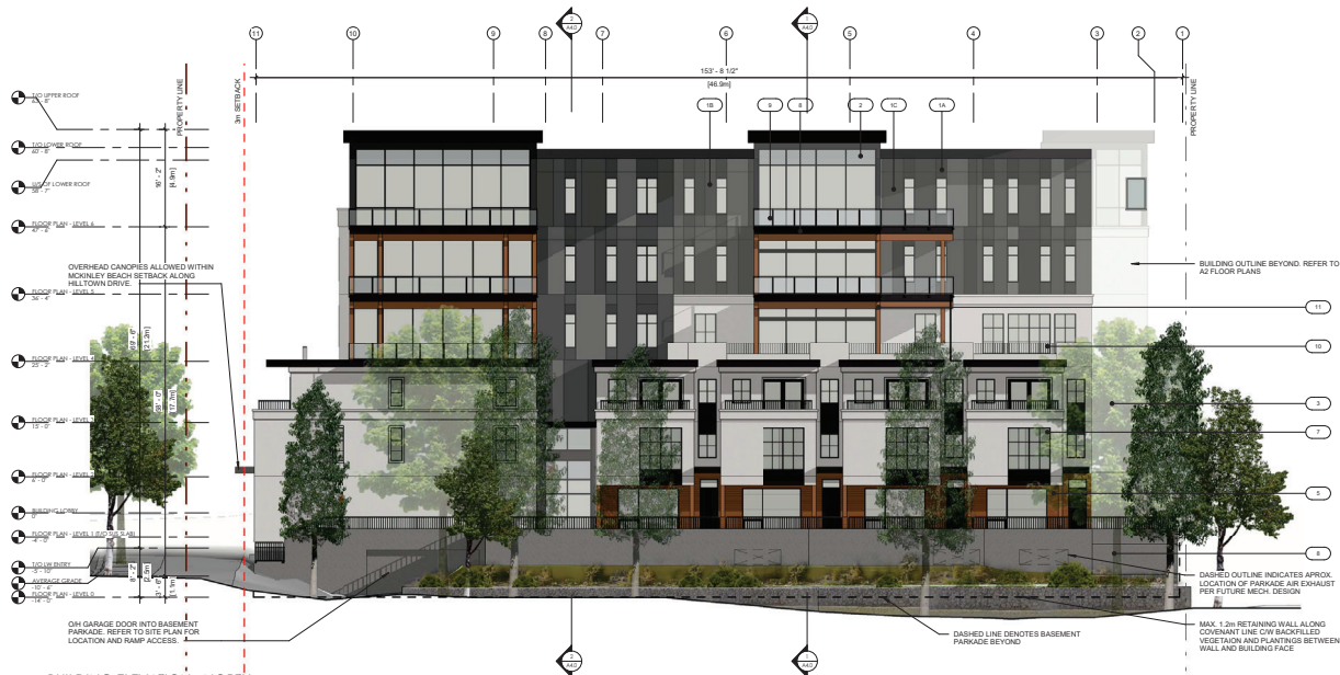
1 BUILDING ELEVATION - NORTH 3/32" = 1'-0"
