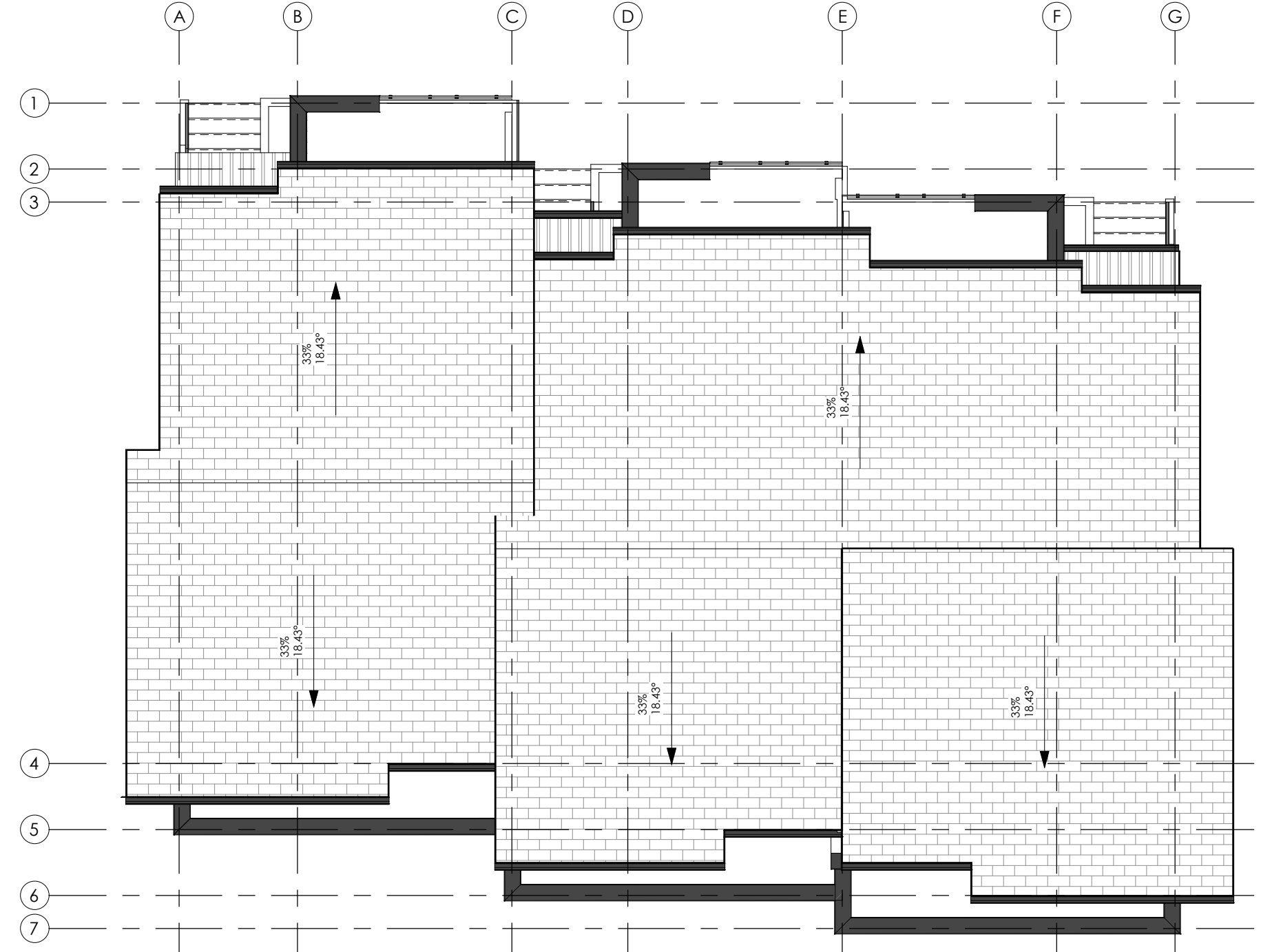
4 ROOF PLAN - BUILDINGS 4, 5, 9 & 10, A1 UNITS 1/8" = 1'-0"
