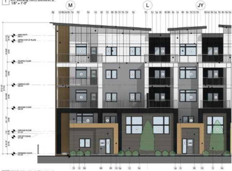
2 SW Building North Elevation A 1/8" = 1'-0"
