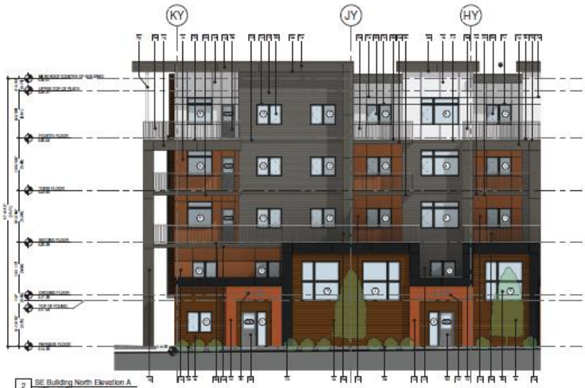
2 SEE Building North Elevation A 3/8" = 1'-0"
