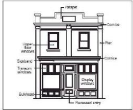
Illustration 4 Typical historic building facade showing major components
