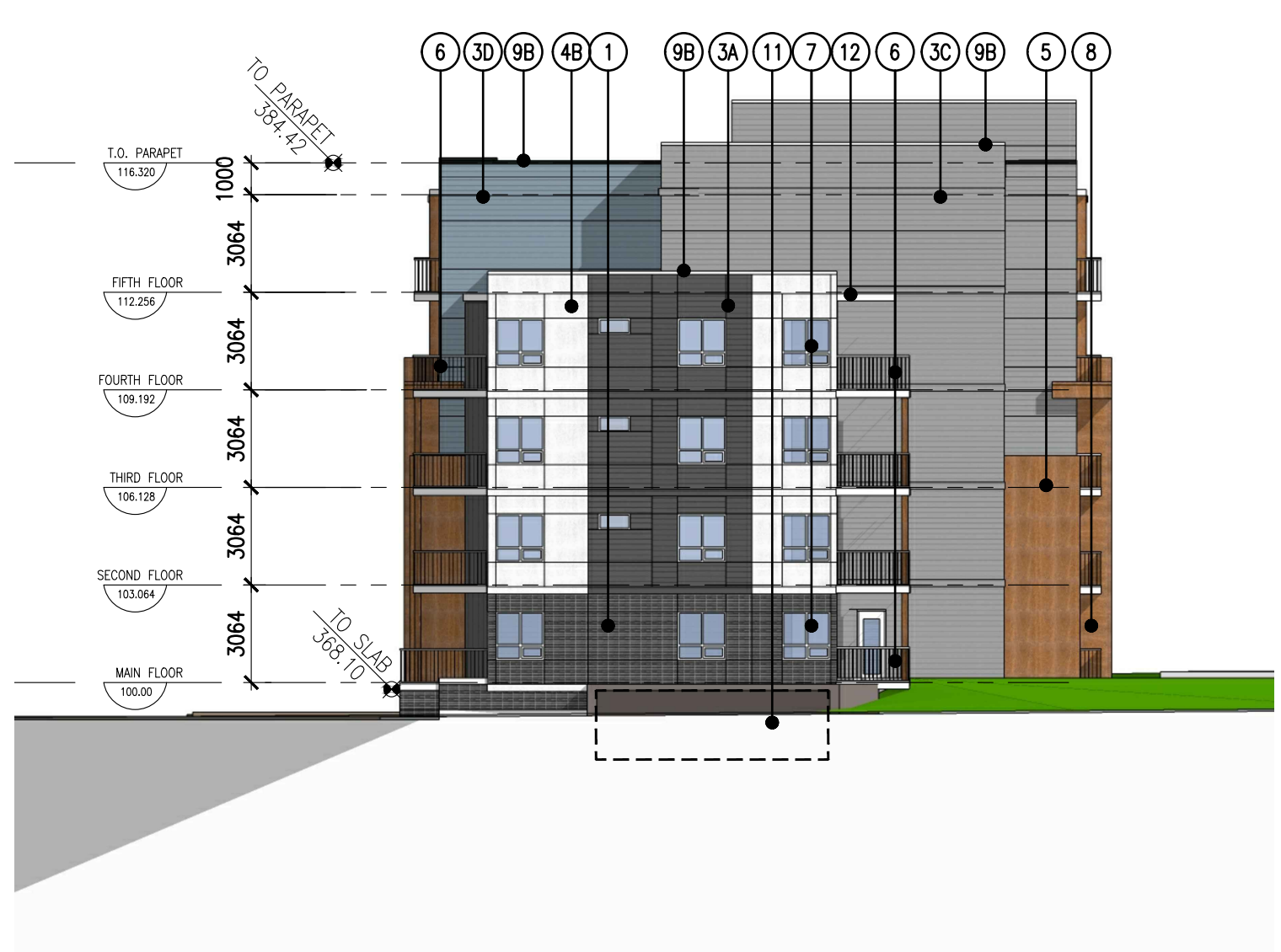
BUILDING 1 WEST ELEVATION SCALE: 1:200
