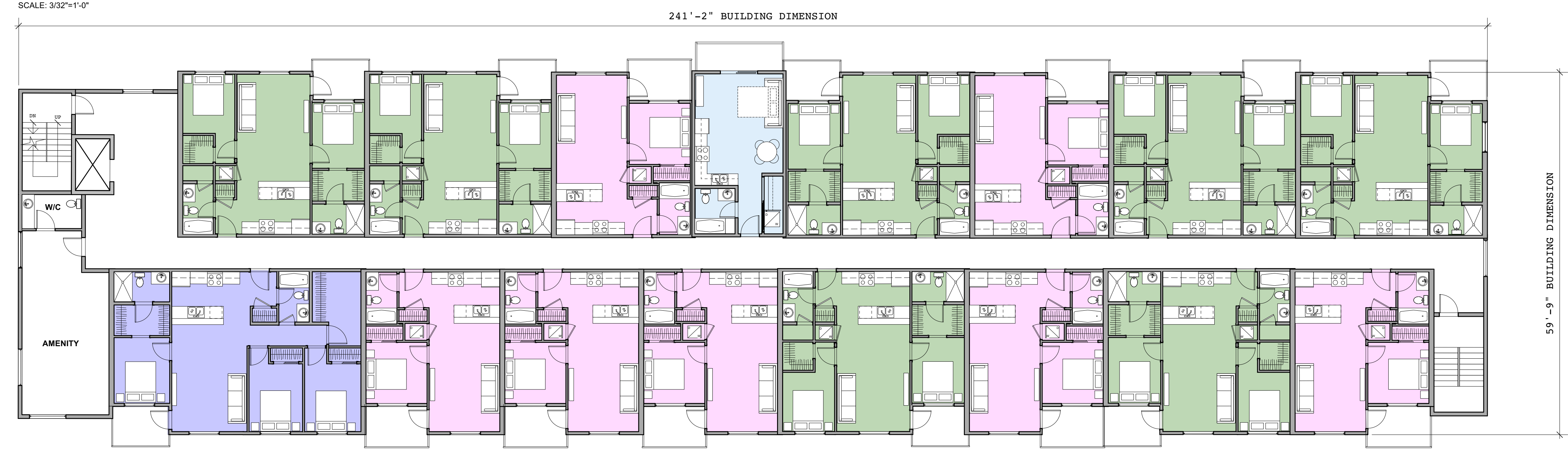
2ND-6TH FLOOR PLAN SCALE: 3/32"=1'-0"
