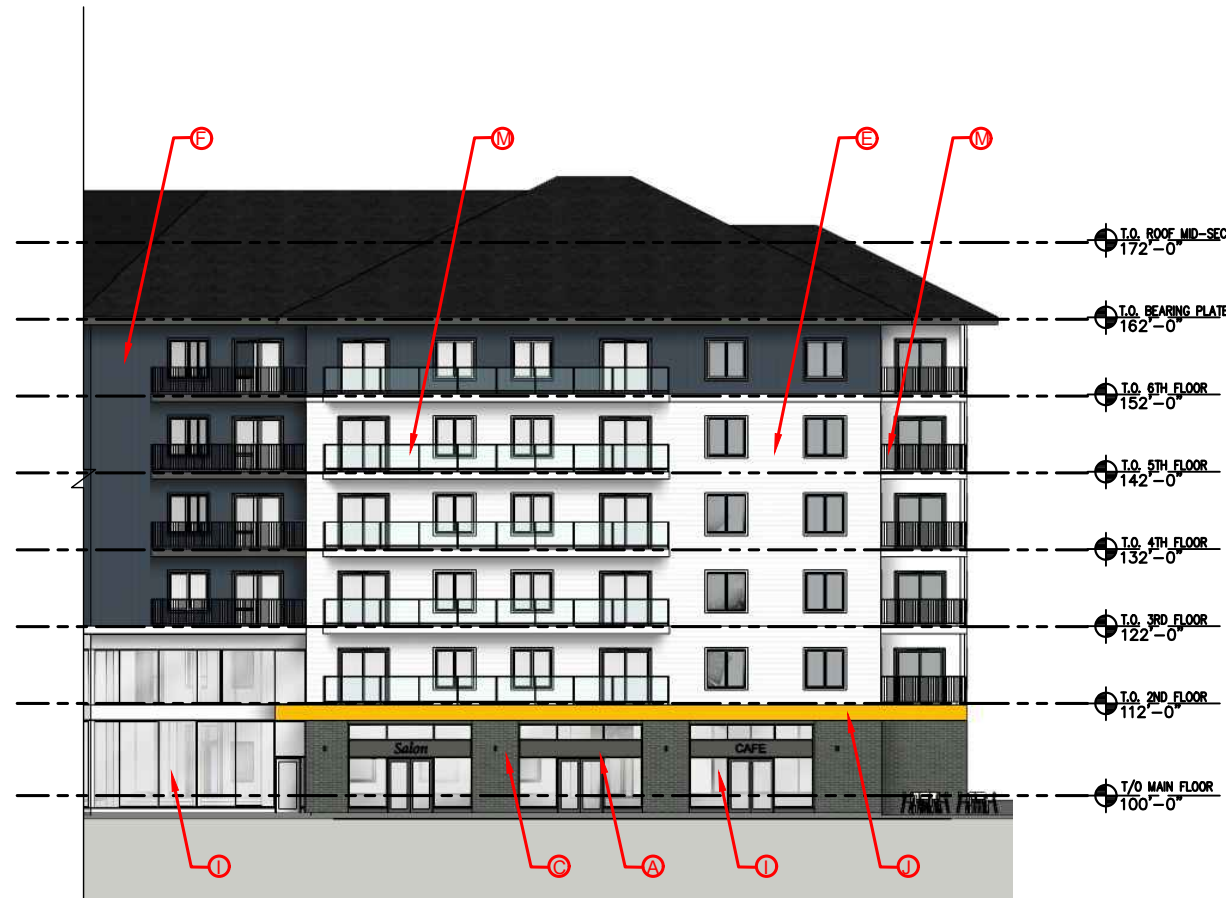
BUILDING 1 (WEST) NORTH ELEVATION SCALE 1:300
