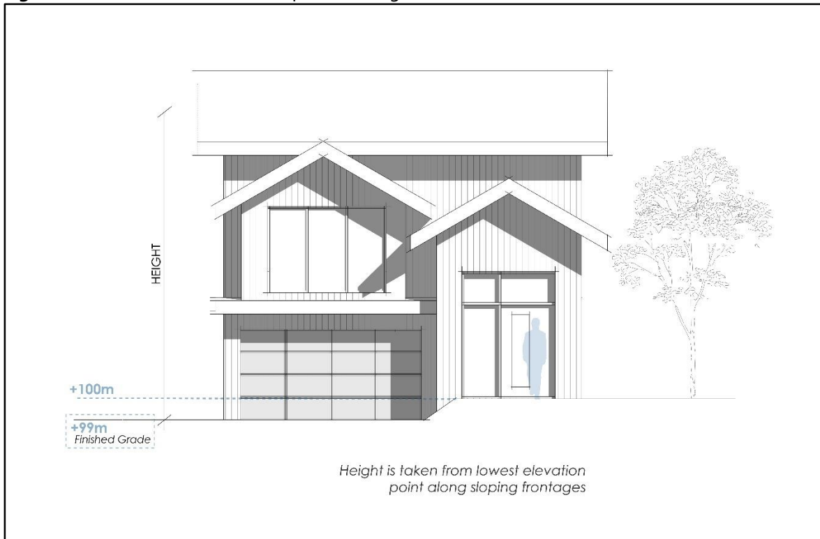
Figure 5.3(c) – Finished Grade: Sloped Fronting Road
