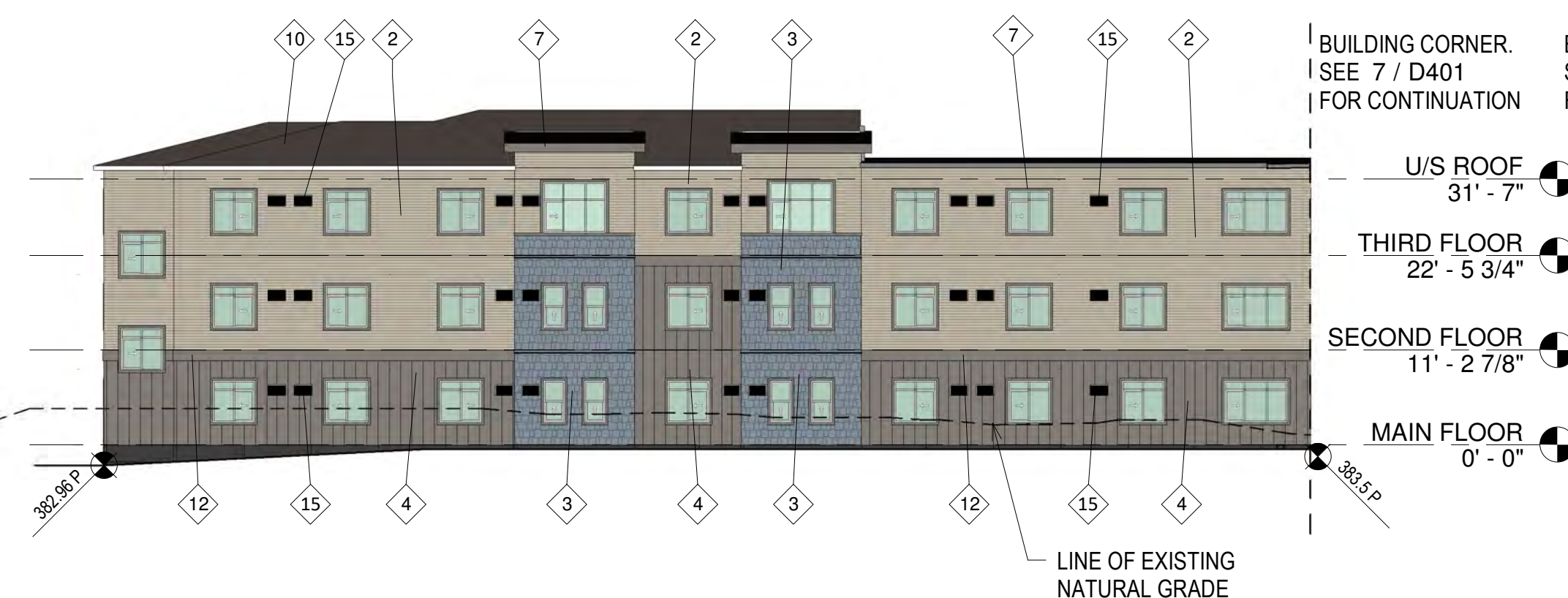
6 PHASE 1 - OPEN COURTYARD NW ELEVATION SCALE: 1 : 200
