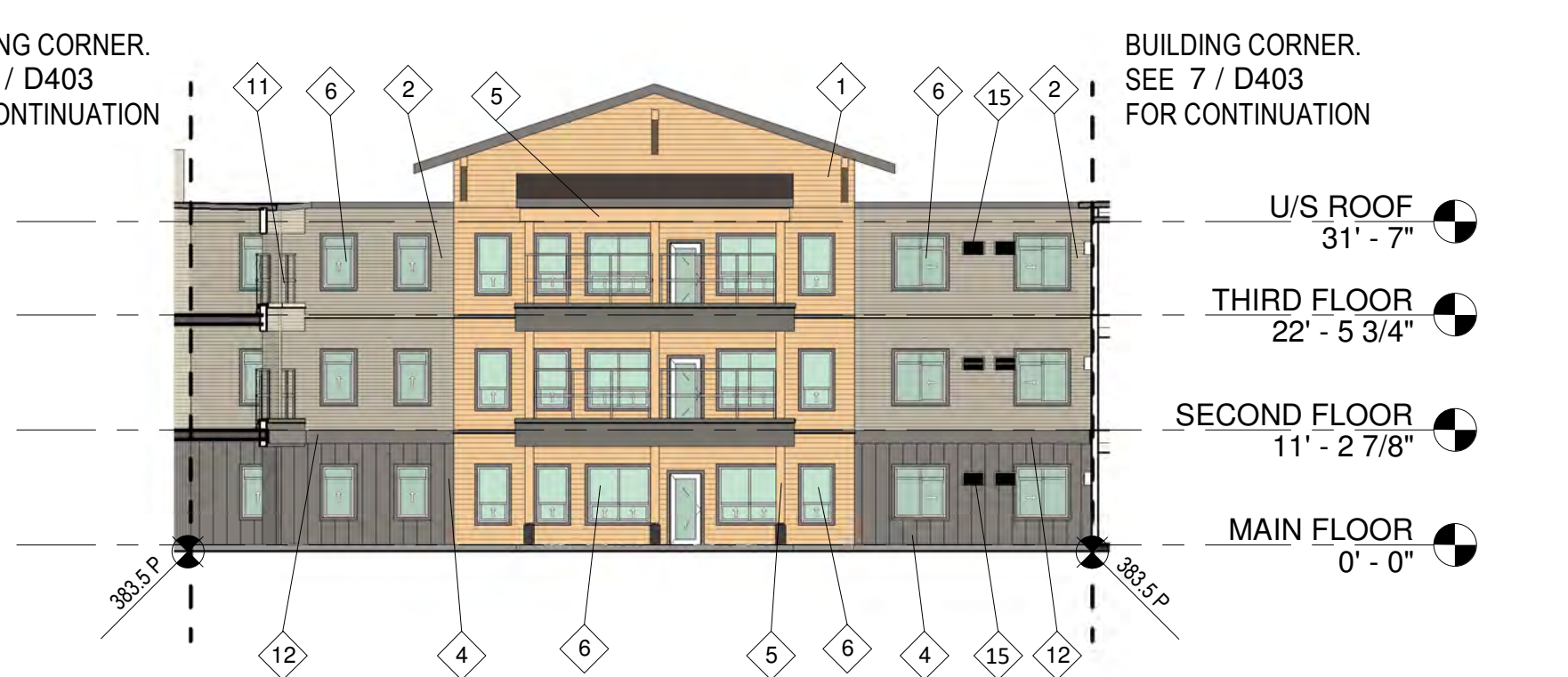
6 PHASE 2/3 - CLOSED COURTYARD NORTH ELEVATION D201 SCALE: 1: 200
