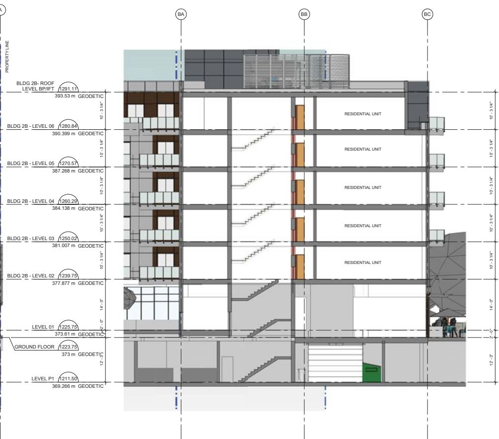
2 A4.05- PH2 BLDG2B - BLDG SECTION 3 Scale: 1/8" = 1'-0"
