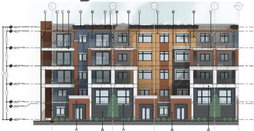
1 Building (A) North Elevation A 1/8" = 1'-0"
