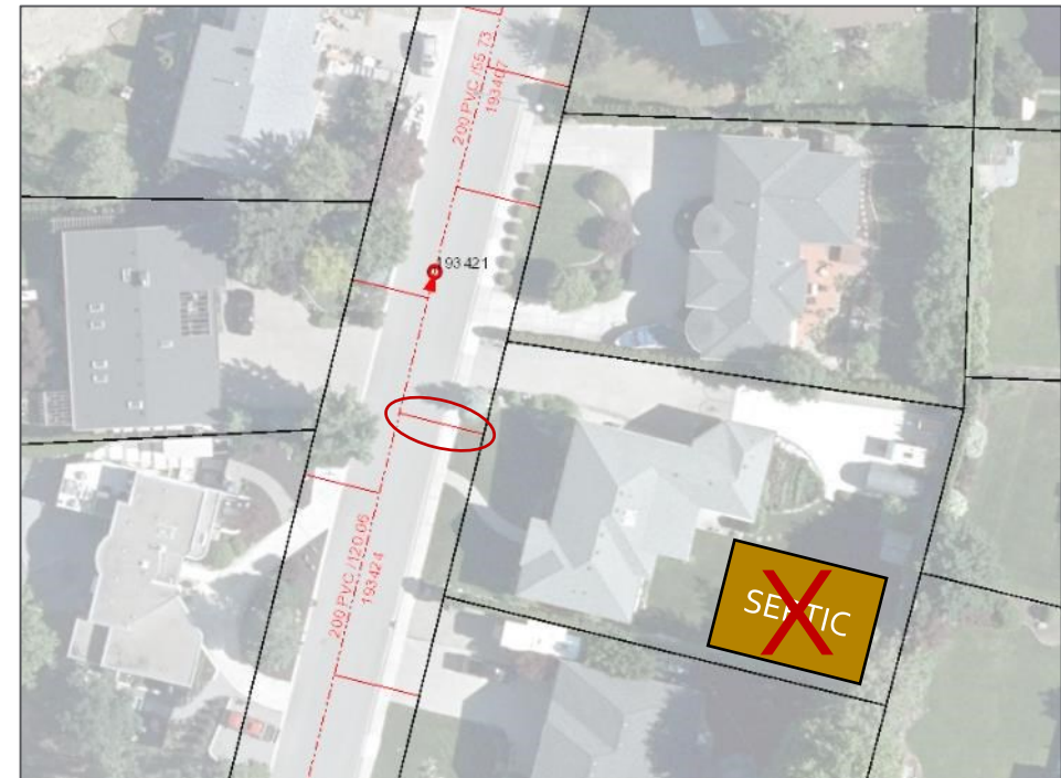
Pre-serviced lots in a sanitary sewer connection area.
