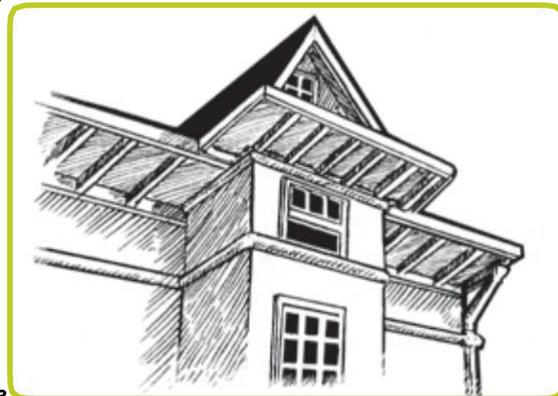
**Figure 23.12: Soffit, Rafter, Rain Water Drainage**
