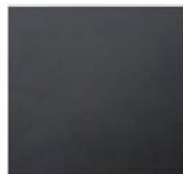
MATERIAL #5 CURTAIN WALL SPANDREL - METAL FINISH: SANDBLAST COLOR: ANTHRACITE - (DARK GREY)
