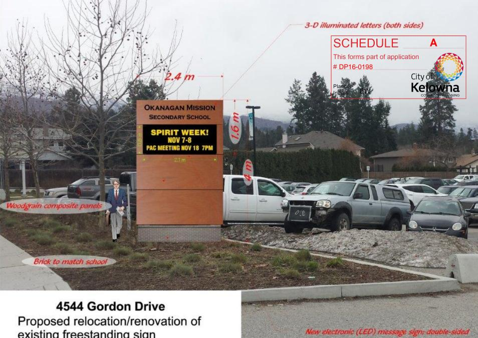
Proposed relocation/renovation of existing freestanding sign Height from Grade = 4.0m Sign area = 3.8m<sup>2</sup> Construction value = \$ 40,000
