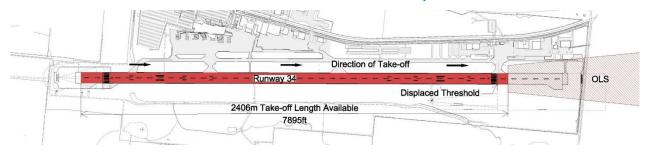
Figure 33: Obstacle Approach Surface for Runway 34 That Can Be Used as a Take-Off Surface for Runway 16
