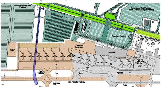
Figure 51: ATB Apron Linear Expansion - Concept 2
