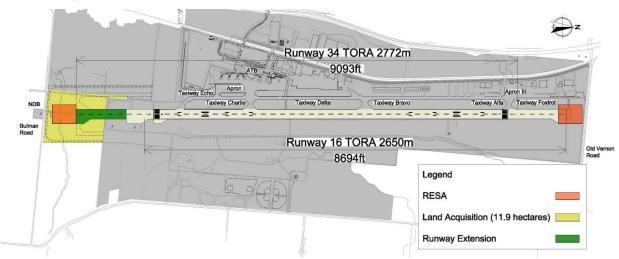
Figure 46: Option 3 for Implementation of Take-off Surface and Increase in TORA
