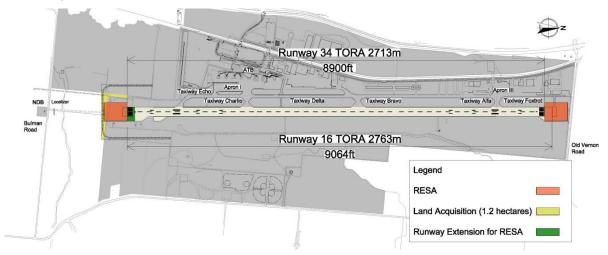
Figure 45: Option 2 for Implementation of Take-off Surface and Increase in TORA
