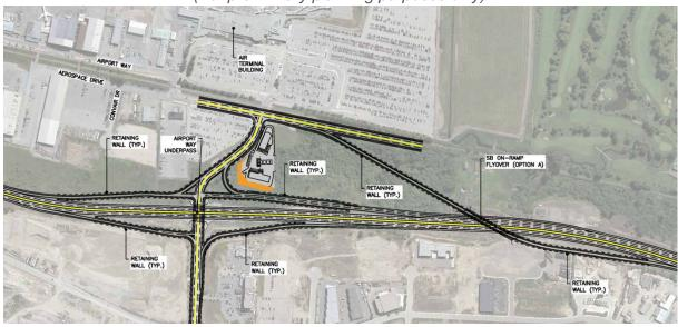
Concept 2 – Southbound Tunnel (Figure 65) replicates the overall intersection configuration described in Concept 1, but moves the southbound traffic flow to a tunnel that would be located below the Airport Way underpass. Southbound traffic would merge with Highway 97.
