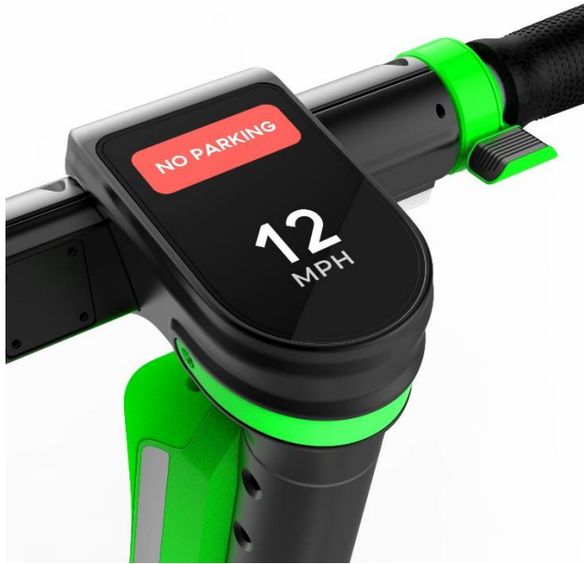
Figure 6 No parking and no riding zones can be indicated by geofencing, smartphone notification, text message and occasionally on the vehicle display itself.
