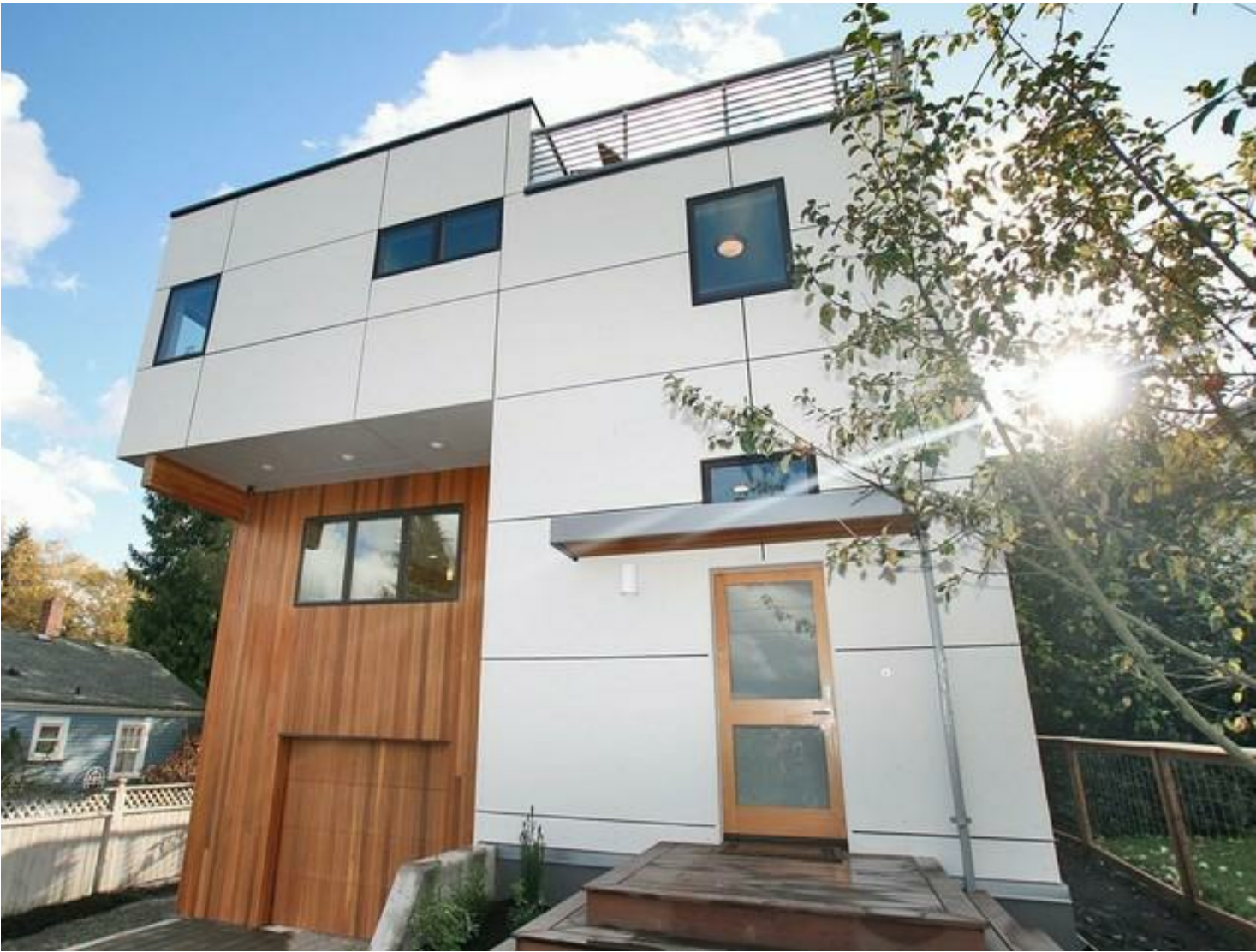
HARDIE REVEAL PANEL (SMOOTH) W/ EASY TRIM REVEAL & PAINTED EXP. FASTENERS; COLOUR PURE WHITE SW 7005 (#2)
