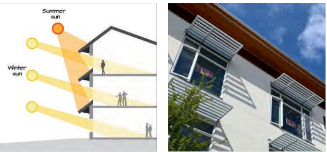
Figure 16: Exterior shading devices can be integrated into a building's southern elevation to block unwanted solar gains and keep indoor temperatures comfortable in warmer months (2.2.1 e).
