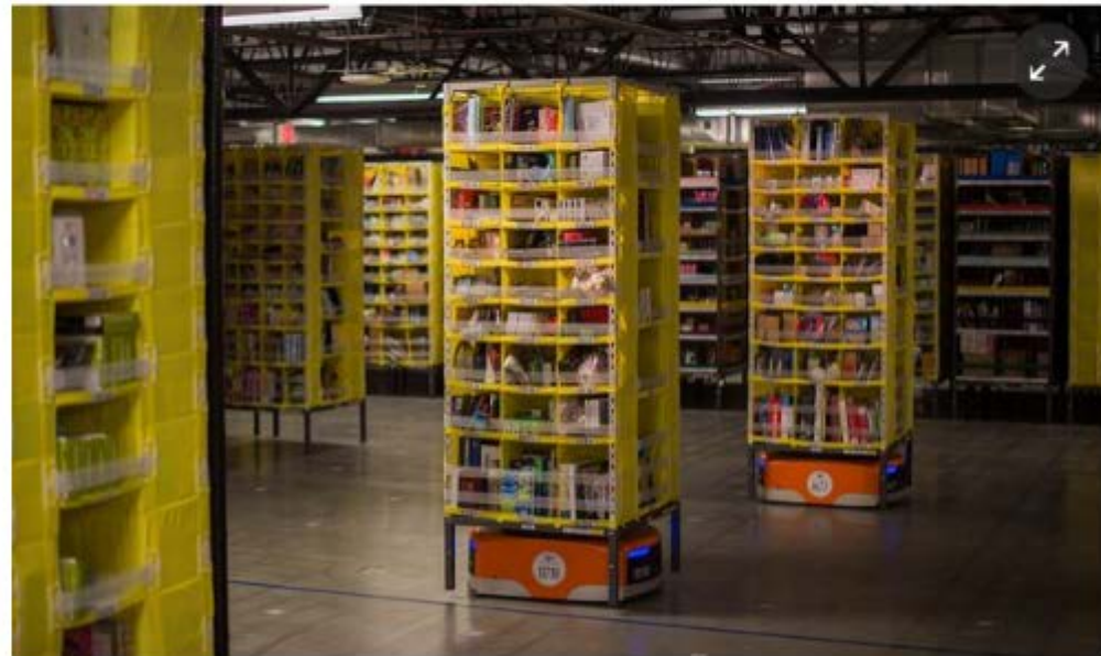
Kiva robots transport goods at an Amazon Fulfillment Center, ahead of the Christmas rush, in Tracy, California in 2014. Photograph: Noah Berger/Reuters
