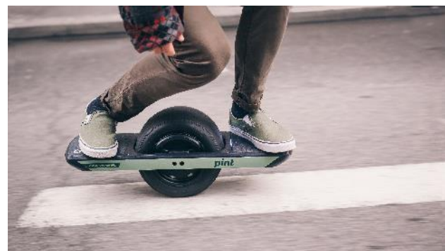
Figure 4 The Onewheel features a self-balancing wheel and footboard. Currently this vehicle is not permitted to operate on roads in Kelowna. 3
