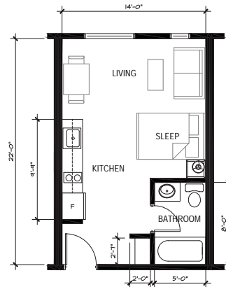
UNIT A FLOOR PLAN SCALE: 1/4" = 1'-0" AREA = 308 SQFT
