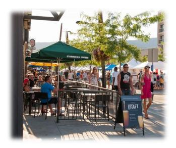
The sidewalk has been divided up into three zones, the frontage zone (adjacent to the buildings), the pedestrian movement zone (in the middle), and the furnishing zone (adjacent to the curb).
