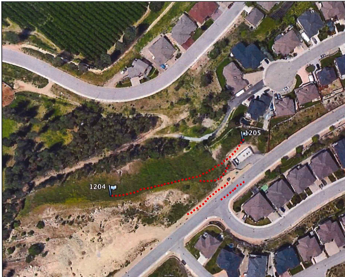
Photo 1: An overview of the approximate location of known and possible tension cracks at the site.
