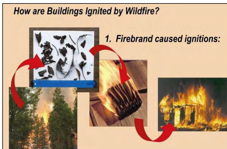
Figure 5. Firebrand caused ignitions: burning embers are carried ahead of the fire front and alight on vulnerable building surfaces.
