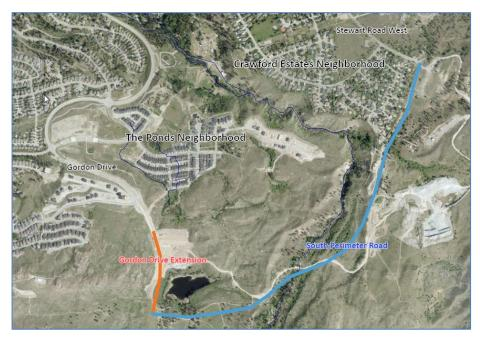
In order for SPR to function as a connected roadway, the existing terminus of Gordon Drive requires an extension of approximately 600-meters to the starting point of South Perimeter Road.¹ The design and construction standard of the Gordon Drive Extension ("GDE"), which has a budget of \$1.663 million, would be similar to the existing standard of Gordon Drive in the Upper Mission.
