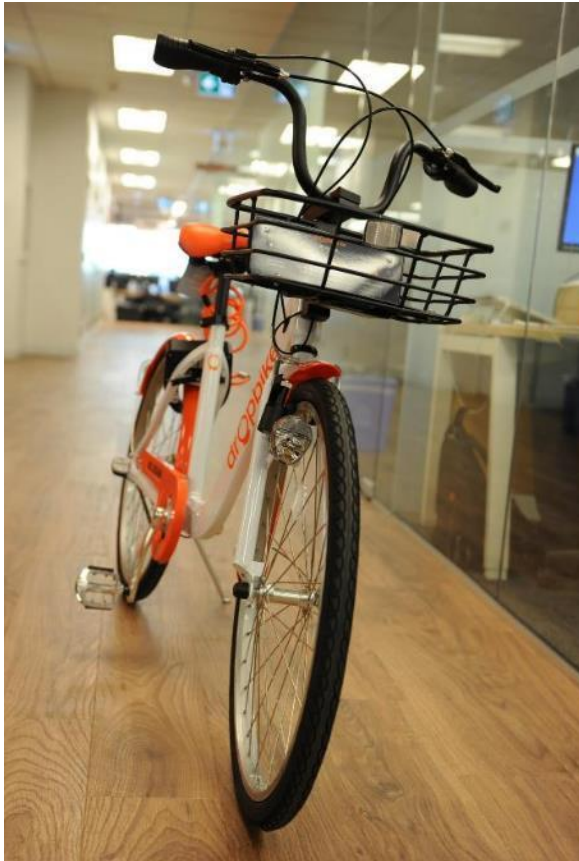
Figure 8 Kelowna's Dropbike fleet attaches the front basket directly to the frame resulting in fewer bikes falling over and improved handling for riders.
