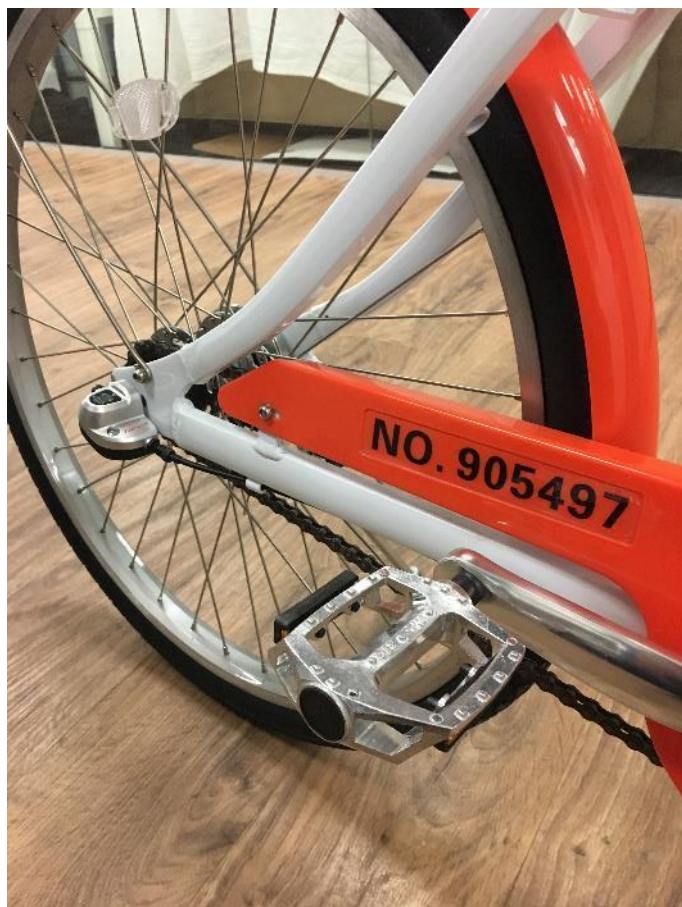
Figure 4 Kelowna's Dropbike fleet is outfitted with internal gears and a drum brake for low maintenance operation.
